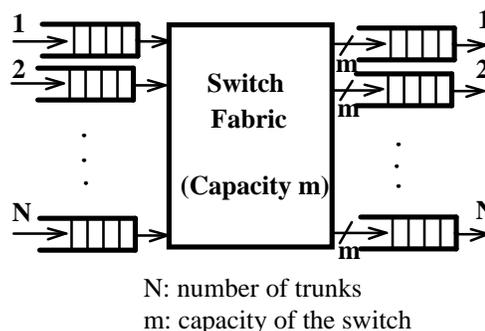
Figure 1. General model of an ATM switch
