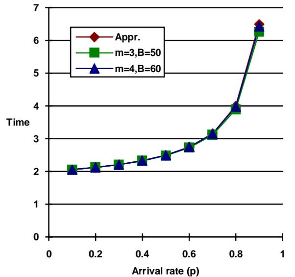
Figure 5. Cell delay from approximation and numerical analysis
