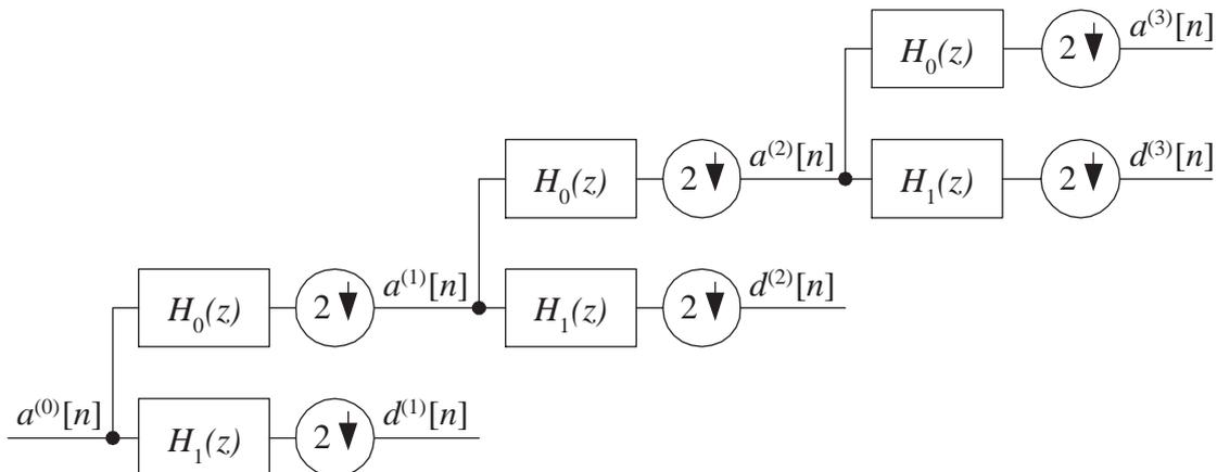
Fig. 2. Wavelet filter bank decomposition
