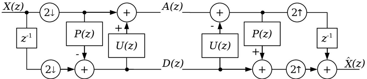
Fig. 5. Filter bank based on the lifting scheme
