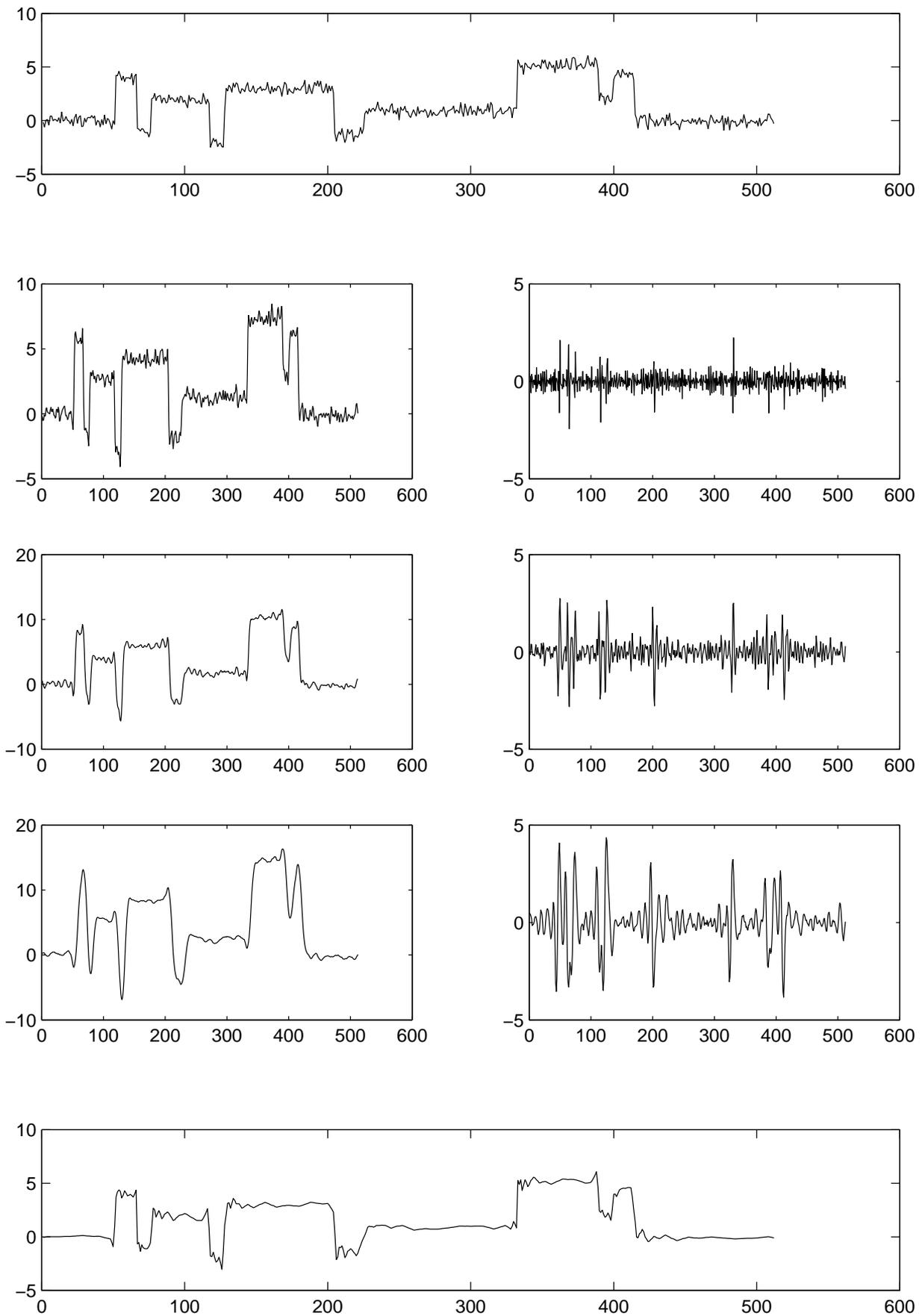
Fig. 4. Noisy Blocks signal denoised using Db3 undecimated wavelet transform
