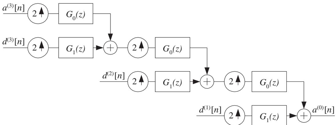
Fig. 3. Wavelet filter bank reconstruction
