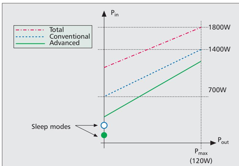
Figure 1. Linear model approximating the relationship between input and output powers of a 3-sector macro base station.
