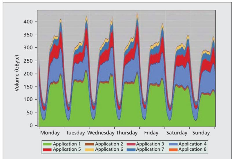
Figure 4. Measured weekly traffic variations of a mobile cellular network [11].
