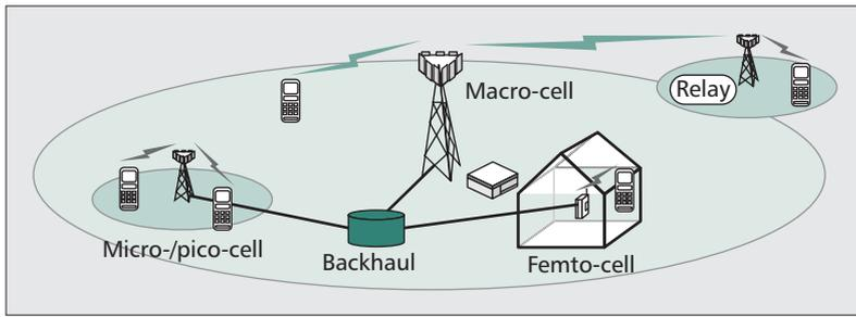
**Figure 3.** Heterogeneous network deployment, consisting of micro-/pico-cells serving hot spot areas, femto-cells for indoor users, and relays for coverage extension.
