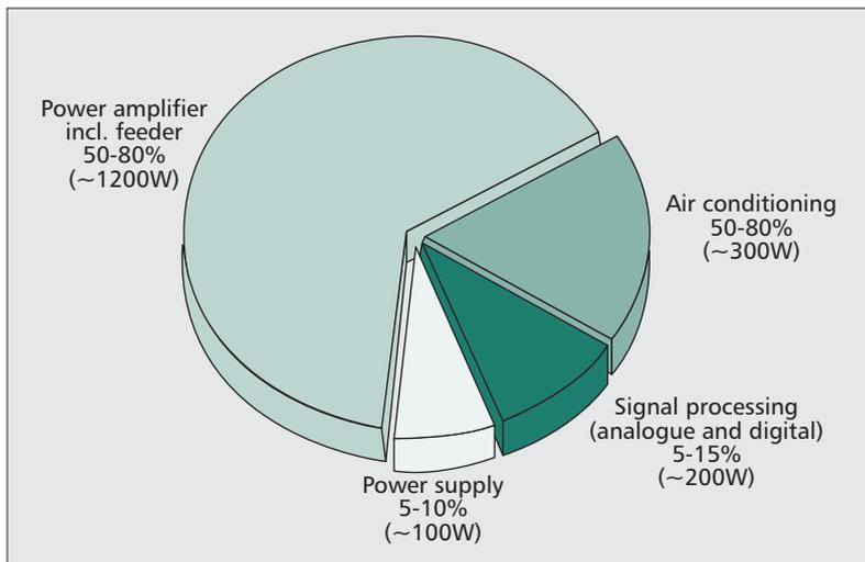
**Figure 2.** Typical power consumption distribution in radio access technology (absolute values relate to the base station of Fig. 1) [5].
