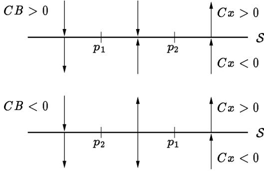
**Fig. 3.** The switch plane  $\mathcal{S}$  and the trajectories for the system in Example 1. If  $CB > 0$ , then there exist sliding modes.
