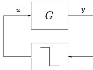
Fig. 1. Relay feedback of linear system  $G$ .
