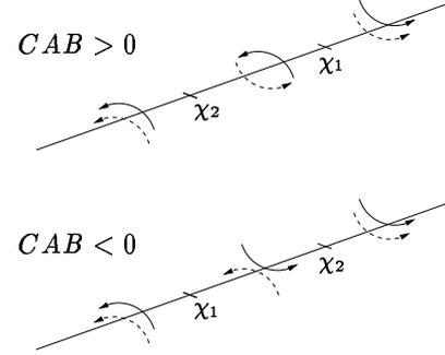
**Fig. 5.** Illustration of Theorem 1. Fast relay switches occur if  $CAB > 0$ .
