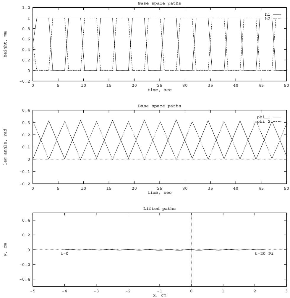
FIGURE 16. Tripod gate for six legged robot. The upper plot shows the motion of the base variables (as a function of time); the lower plot shows the  $xy$  motion of the robot (the  $y$  scale is enlarged to show the rocking motion).
