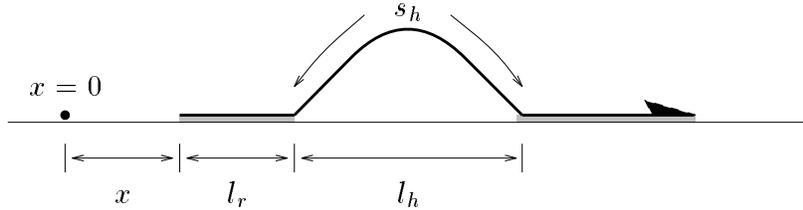
FIGURE 5. Simple model for an inchworm robot
