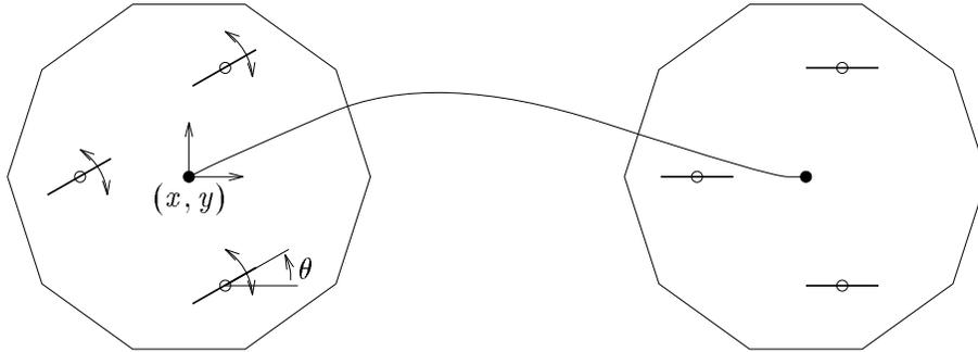
FIGURE 3. Wheeled mobile robot which maintains fixed orientation.
