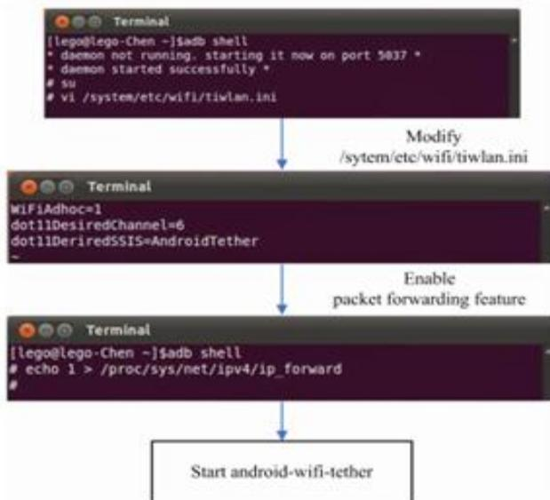
**Figure 4. Configuration steps for AdHoc networking**
