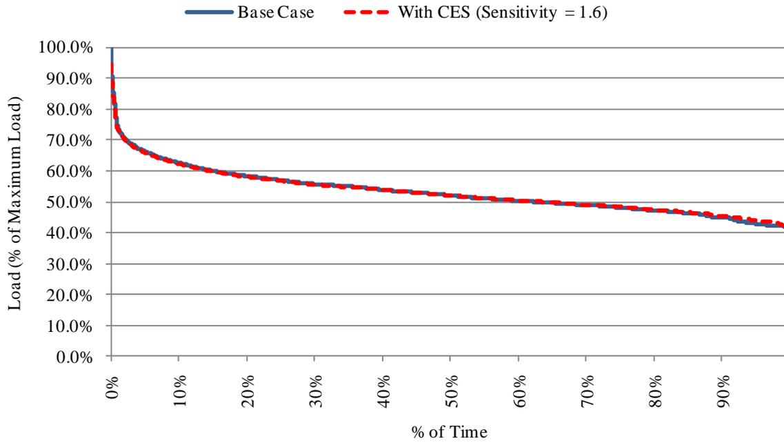
**Figure 27 : Load duration curves for base case and CES case (sensitivity = 1.6).**
