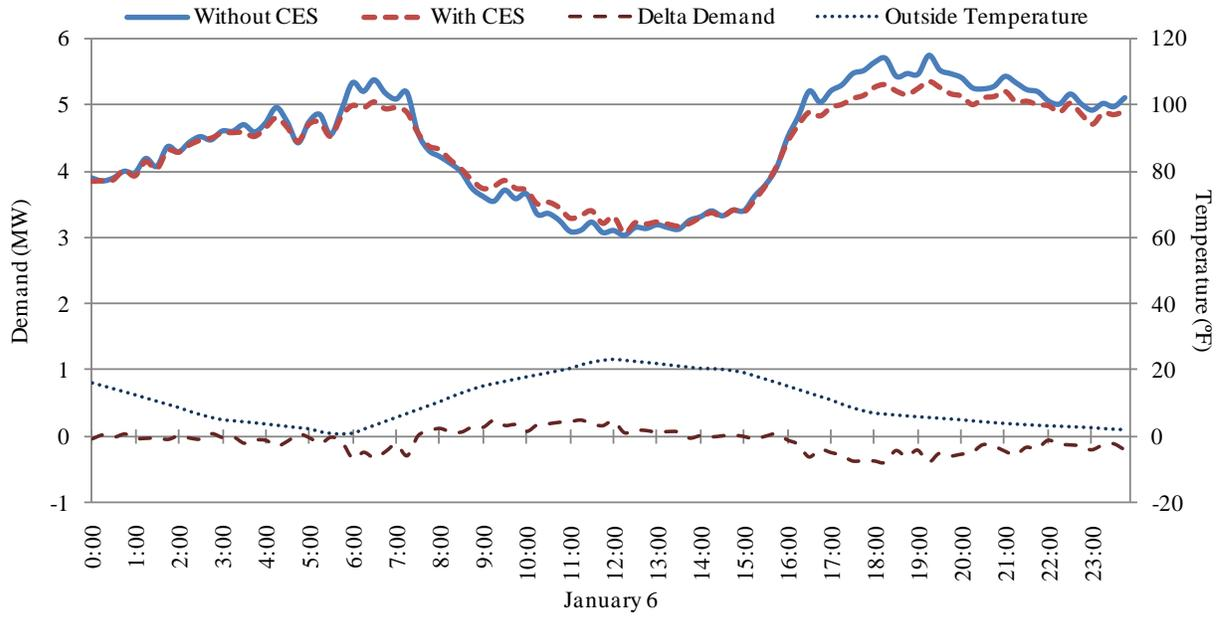
Figure 21 : Comparison of substation demand with and without CES on a cold day.
