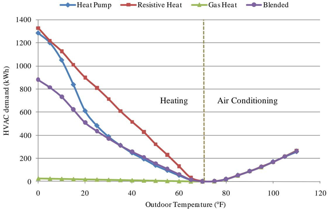
**Figure 6 : Load demand as a function of air temperature on 100 simulated homes.**
