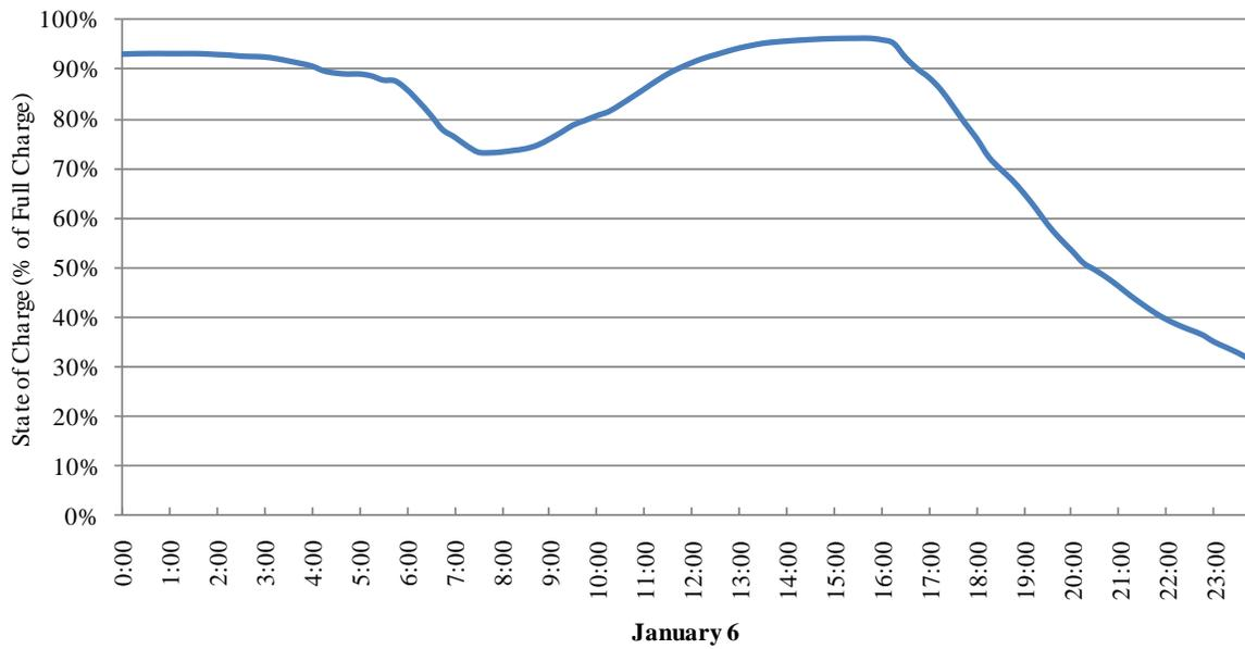
Figure 22 : Total energy in the CES system as a percentage of maximum capacity on a cold day.
