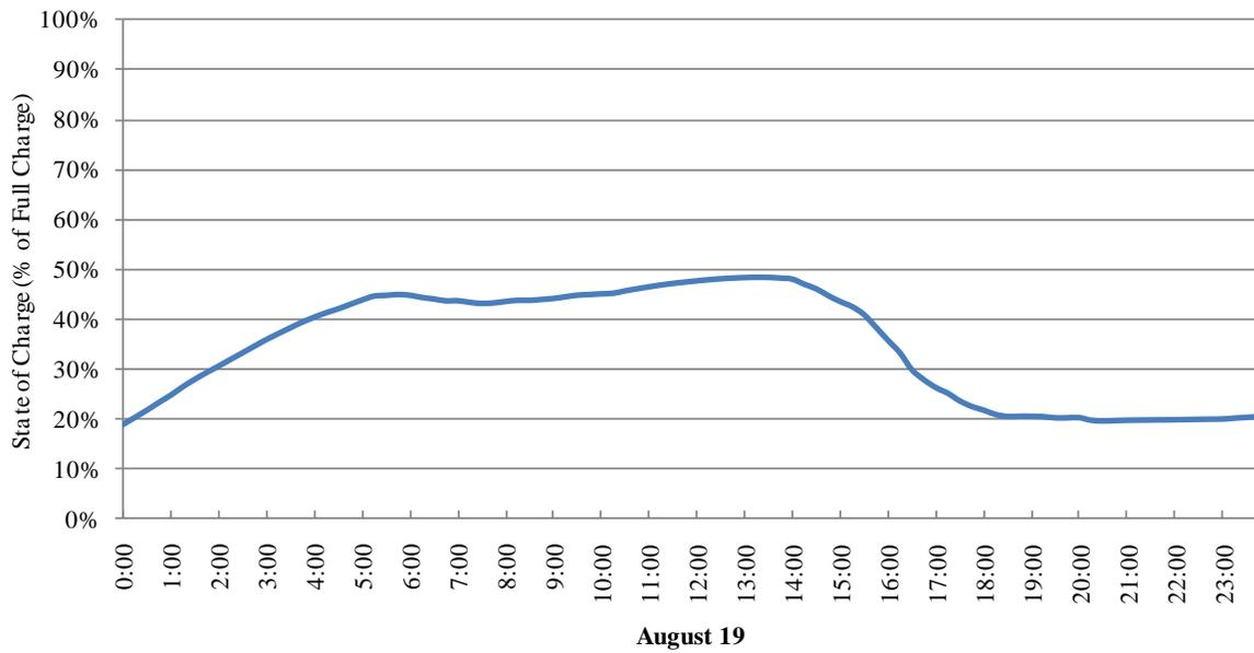
Figure 24 : Total energy in the CES system as a percentage of maximum capacity on a mild temperature day.
