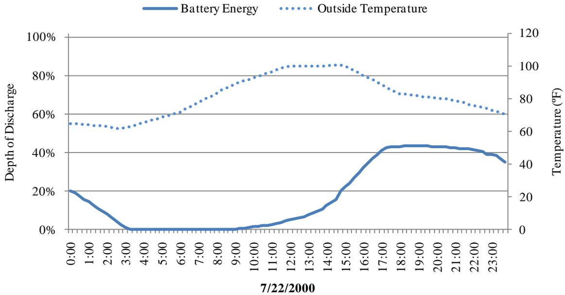
**Figure 16 : Depth of discharge of the battery on a warm day.**
