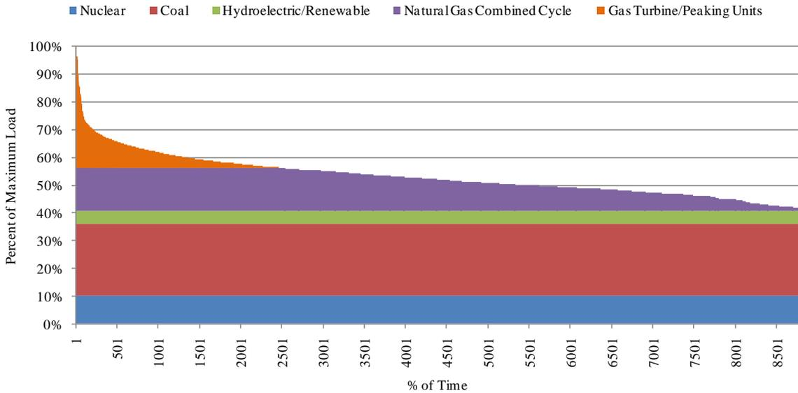
**Figure 30 : Dispatch of generation for base case of Chapter 5.1 using U.S. generational mix.**
