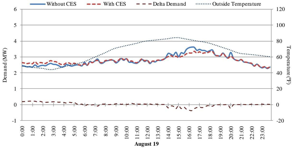
Figure 23 : Comparison of substation demand with and without CES on a mild temperature day.
