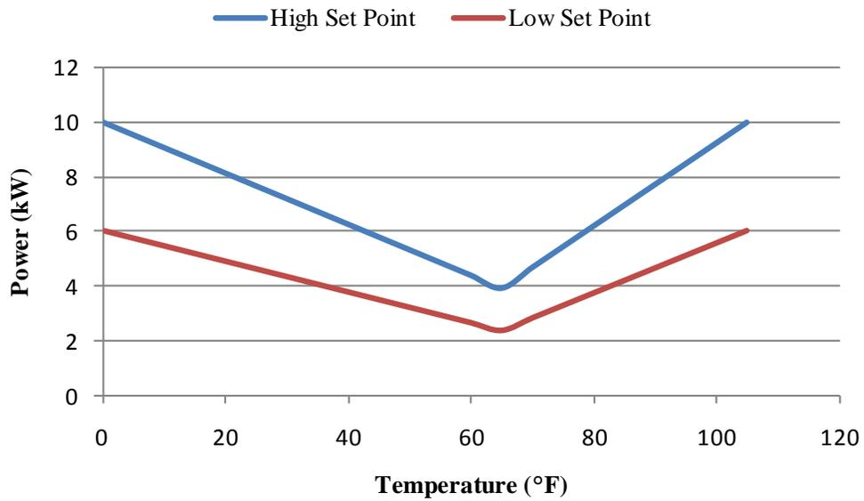
Figure 9 : Example of proposed, temperature dependent set points for CES controller.
