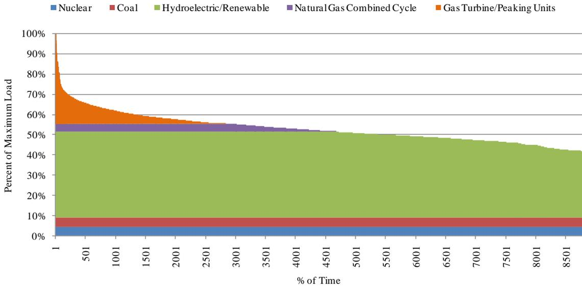
**Figure 29 : Dispatch of generation for base case of Chapter 5.1 using Washington St. generational mix.**
