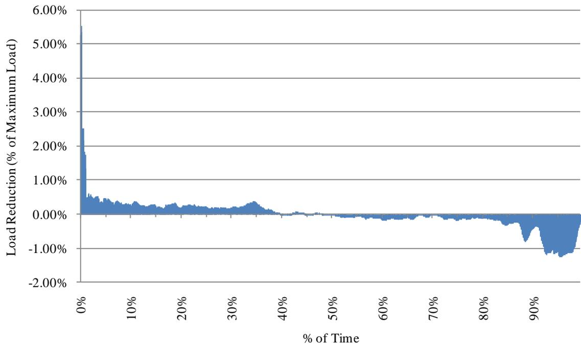
**Figure 28 : Difference between load duration curves for base case and CES case.**
