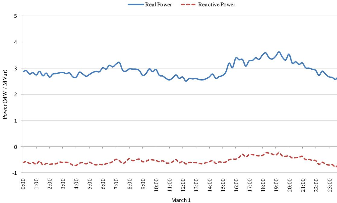
**Figure 20 : Example 24 hour load demand for modified feeder R1-12.47-4 without CES.**
