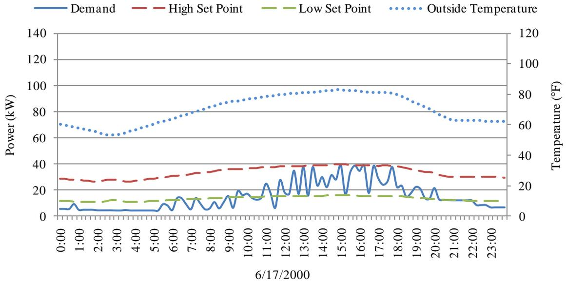
Figure 18 : Average temperature day load demand with battery control.
