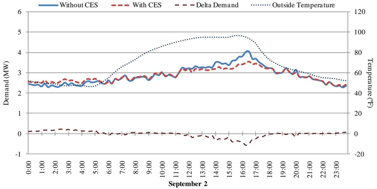
Figure 25 : Comparison of substation demand with and without CES on a warm day.
