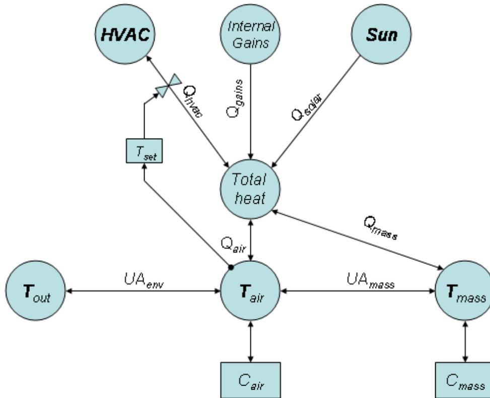
Figure 1 : Flow diagram of ETP model [26].
