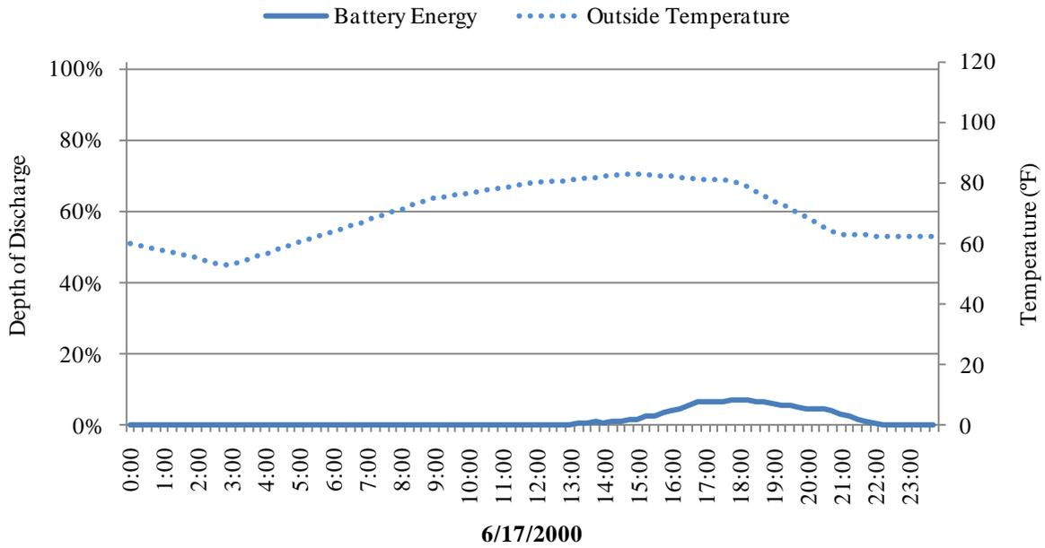
Figure 19 : Depth of discharge of the battery on an average temperature day.
