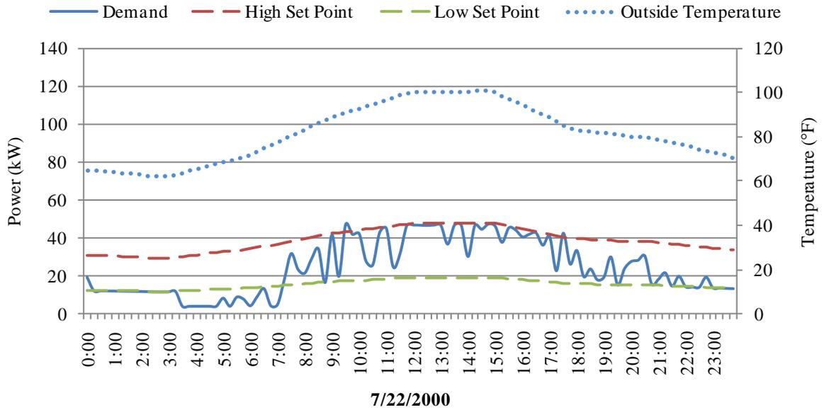
Figure 15 : Power demand on high temperature day while using CES device.
