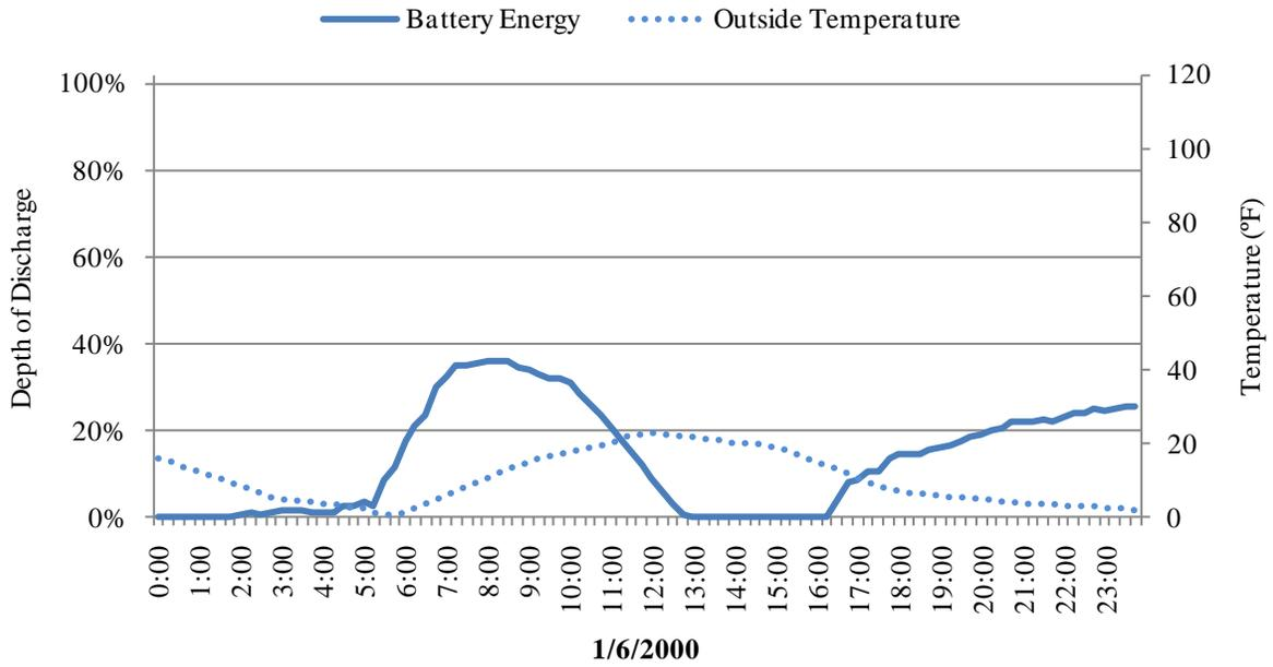
Figure 14 : Depth of discharge of the battery on a cold day.
