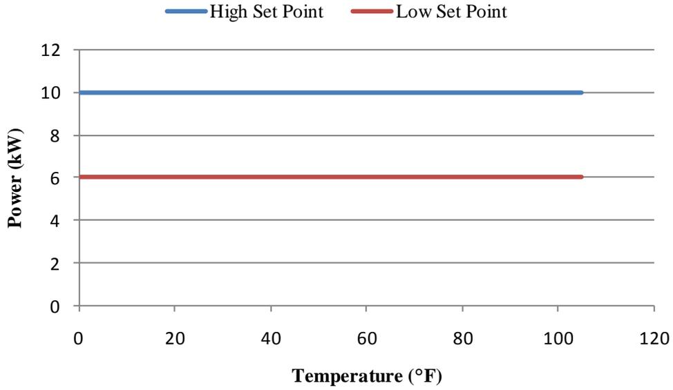
Figure 8 : Example of un-controlled set points for CES controller.
