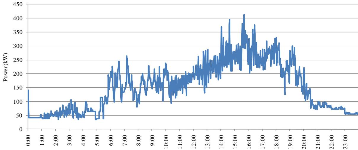
**Figure 4 : Load shape of an aggregate of 100 homes.**
