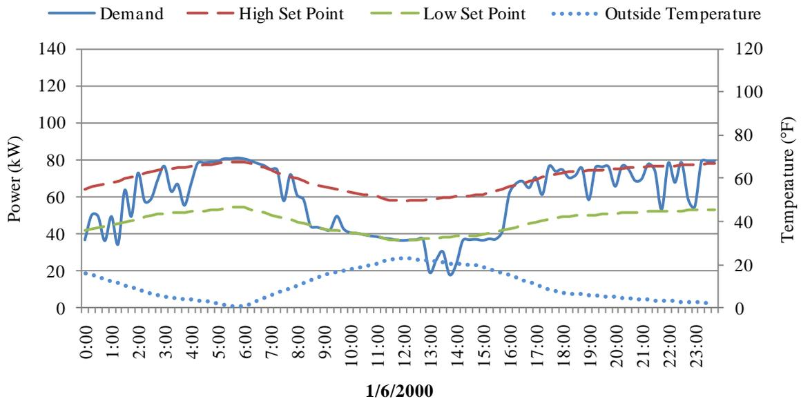
**Figure 13 : Power demand on low temperature day while using CES device.**
