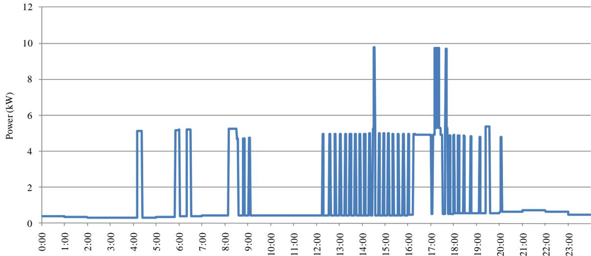
**Figure 2 : Load shape of a single home.**
