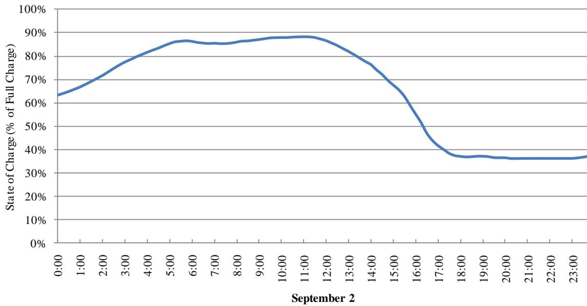
Figure 26 : Total energy in the CES system as a percentage of maximum capacity on a warm day.
