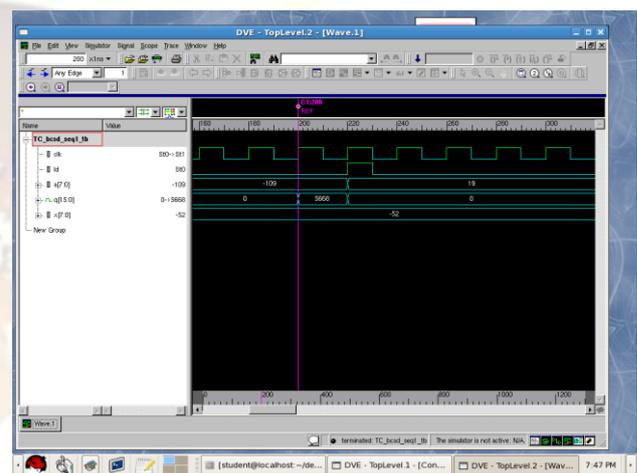
Figure 2. Simulation results of BCSD multiplier.
