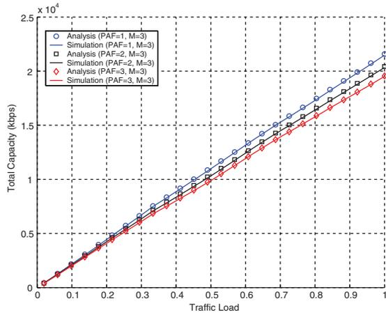
**Fig. 5.** Total capacity of a cell of the proposed SqFR with  $M$  of 3 under heterogeneous traffic condition.
