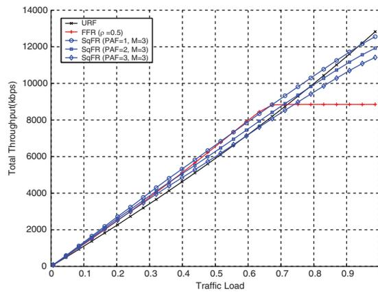
**Fig. 9.** Total throughput of a cell under heterogeneous traffic condition for SqFR with  $M$  of 3, UFR, and FFR.
