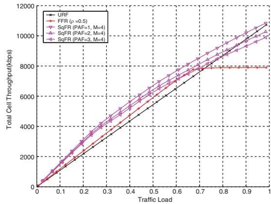
**Fig. 7.** Total throughput of a cell under homogeneous traffic condition for SqFR with  $M$  of 4, UFR, and FFR.
