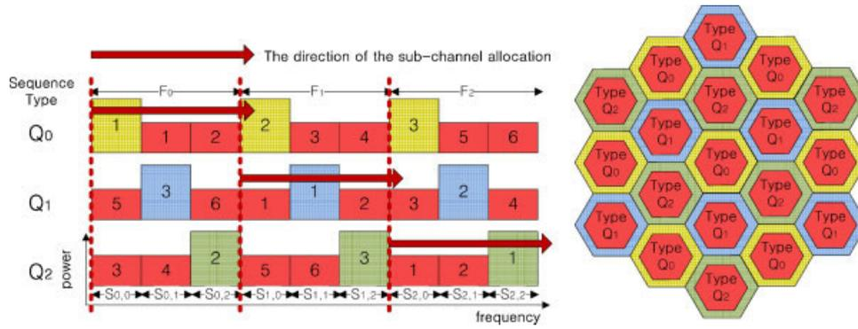
Fig. 2. An example of SqFR with the size of sub-channel sets,  $M$ , of 3.
