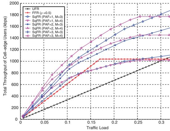
**Fig. 8.** Total throughput of cell-edge users under homogeneous traffic condition.
