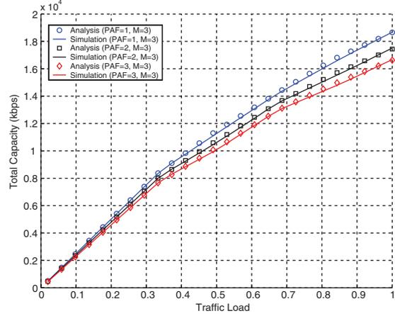
**Fig. 4.** Total capacity of a cell of the proposed SqFR with  $M$  of 3 under homogeneous traffic condition.
