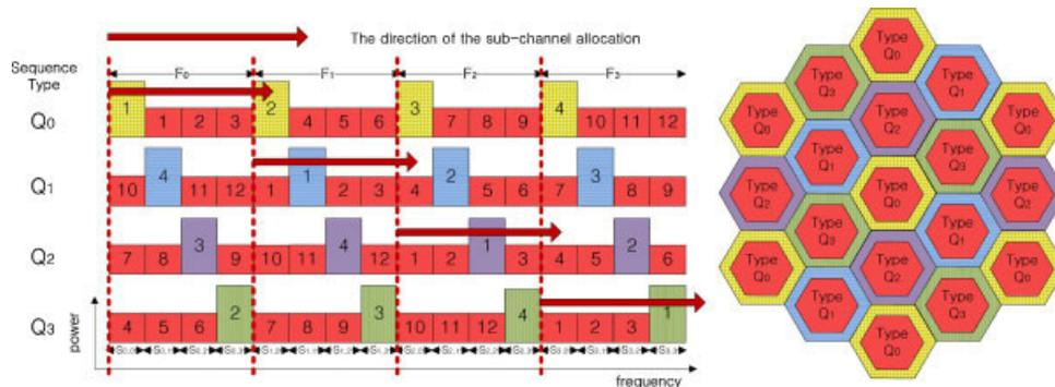
Fig. 3. An example of SqFR with the size of sub-channel sets,  $M$ , of 4.
