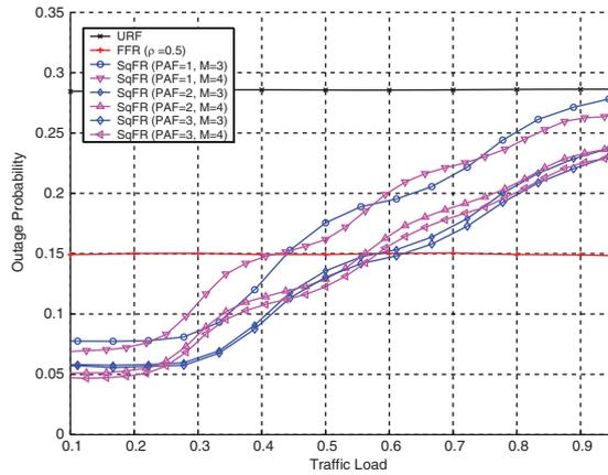
Fig. 12. Outage probability with  $\text{CINR}_{\text{out}} = 0\text{dB}$  under homogeneous traffic condition.
