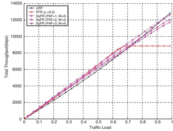
**Fig. 10.** Total throughput of a cell under heterogeneous traffic condition for SqFR with  $M$  of 4, UFR, and FFR.
