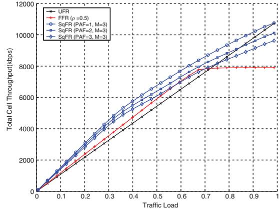
**Fig. 6.** Total throughput of a cell under homogeneous traffic condition for the proposed SqFR with  $M$  of 3, UFR, and FFR.
