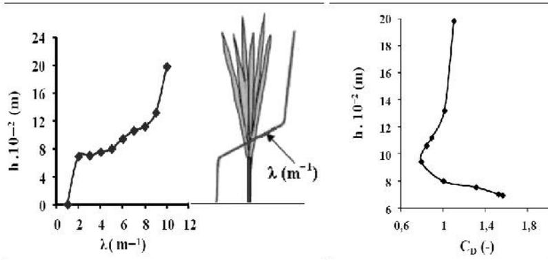
**Figure 3:** Profiles of vegetation density  $\lambda$  (left) and drag coefficient  $C_D$  (right): (the case of 280 plants)
