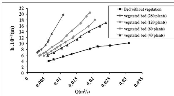
Figure 2: Water depth-discharge relationship for flow through different vegetation densities
