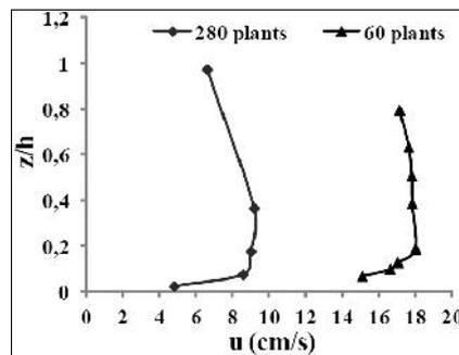
Figure 5: Profile of mean velocity for 280 and 60 plants ( $Q = 0.0128 \text{ m}^3/\text{s}$ )
