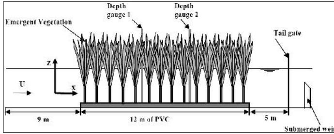
Figure 1: Experimental set-up in the flume with vegetation
