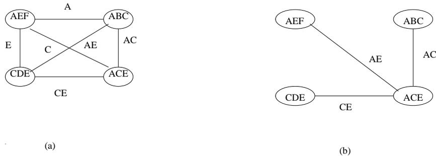
Figure 7: A dual-constraint graph and its join tree.
