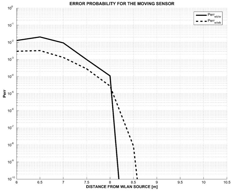
Figure 16: Error probability of WLAN and WLAN+Bluetooth classes for the cooperative scenario.
