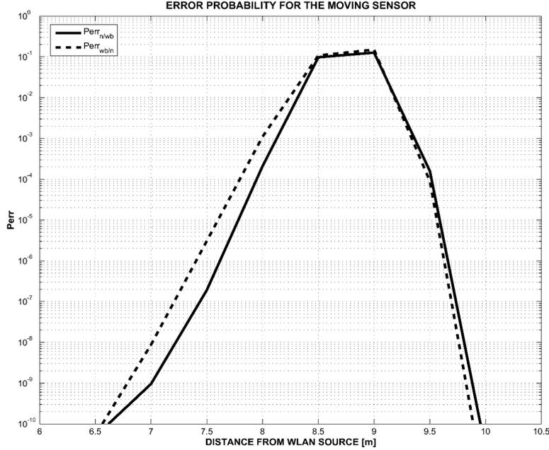
Figure 15: Error probability of WLAN+Bluetooth and Noise classes for the stand alone scenario.
