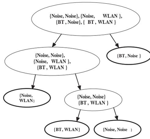
Figure 8: The first binary decision tree used by each sensor.
