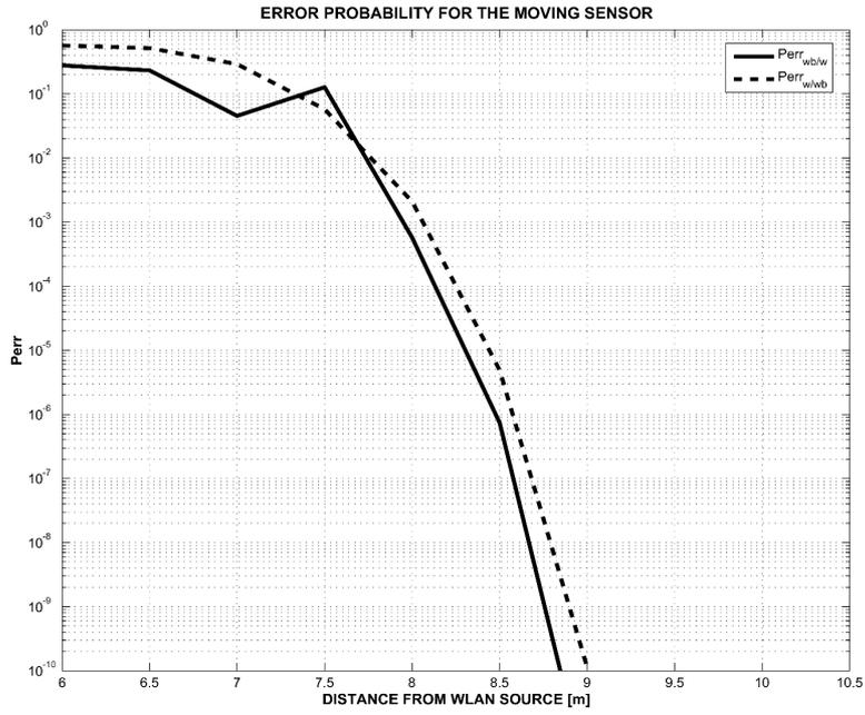
Figure 17: Error probability of WLAN and WLAN+Bluetooth classes for the stand alone scenario.
