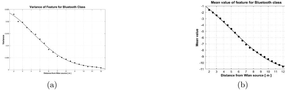
Figure 13: Parameters of feature (after KL reduction) for bluetooth class in relation to user's distance from WLAN source. Variance (a), mean value (b).
