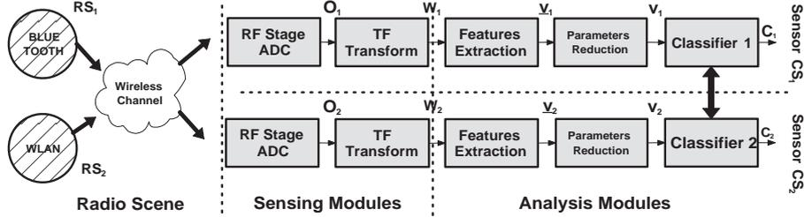
Figure 3: Logical Architecture of two Cooperative Sensors.
