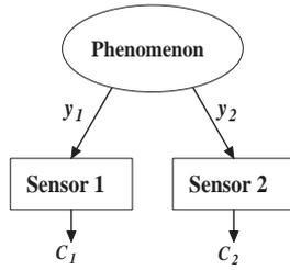
Figure 10: Parallel decision performed by two sensors of a binary phenomenon.
