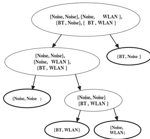
Figure 9: The second binary decision tree used by each sensor.
