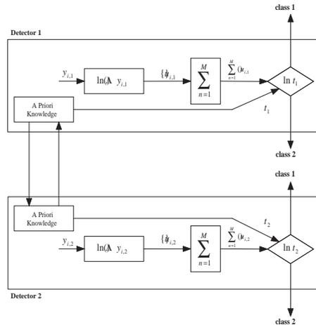
Figure 11: Structure of a distributed detection system
