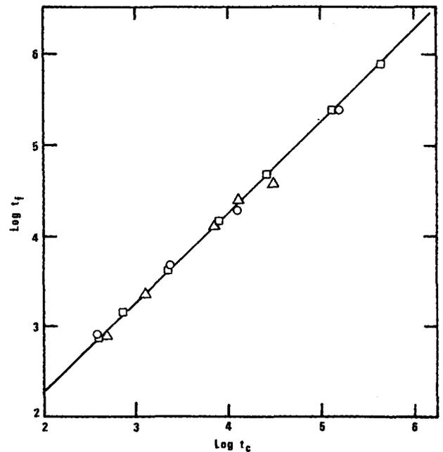
Fig. 2. Log time to failure ( $t_f$ ) vs log of the critical time ( $t_c$ ) at 296K: triangles—sample D ( $M_w = 99,000$ ), circles—sample A ( $M_w = 160,000$ ), and squares—a third linear polyethylene (not described in the text) with an  $M_w = 192,000$  but same  $M_n$  as the other two samples.
