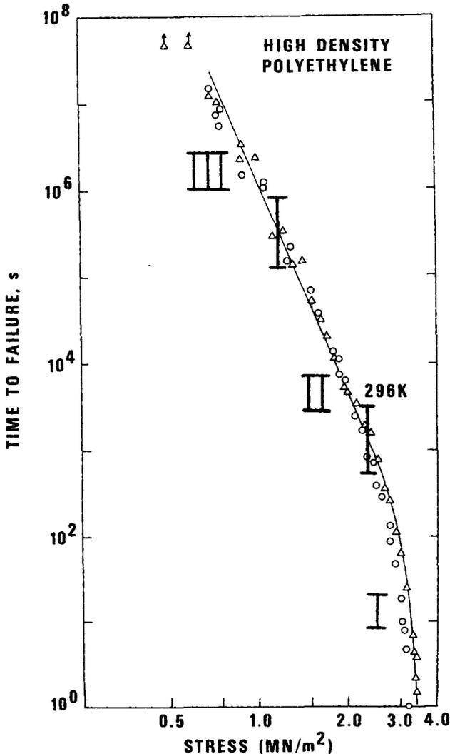
Fig. 1. Log time to failure in uniaxial extension vs log stress for two samples of high density polyethylene: circles—sample A ( $M_w = 160,000$ ), triangles—sample D ( $M_w = 99,000$ ). The points with arrows represent specimens still under test.
