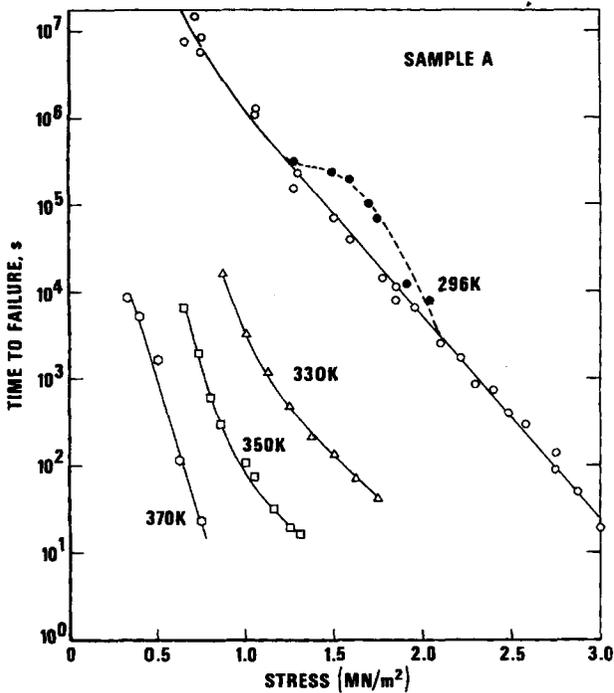
Fig. 5. Log time to fail vs applied stress for sample A. The solid points at 296K correspond to the time to fracture after necking has occurred.
