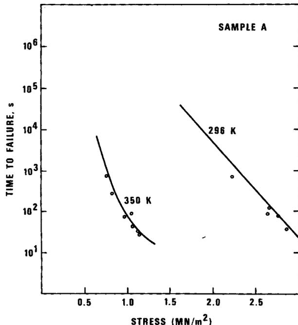
Fig. 3. Prediction of time to failure for a static load based on constant rate of loading experiments. Solid lines represent data for time to fail vs static load; circles—predicted values calculated from Eq 6.
