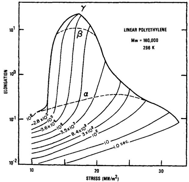
Fig. 7. Log elongation vs applied stress in terms of isochrones for the uniaxial creep of sample A. For an explanation of lines  $\alpha$ ,  $\beta$ , and  $\gamma$ , see the text.
