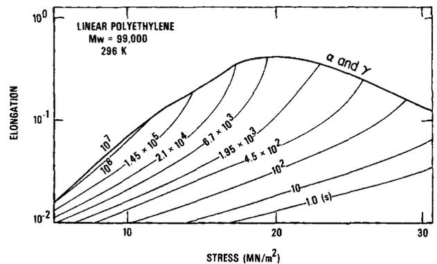
Fig. 8. Log elongation vs applied stress in terms of isochrones for the uniaxial creep of sample D. For an explanation of lines  $\alpha$  and  $\gamma$ , see the text.
