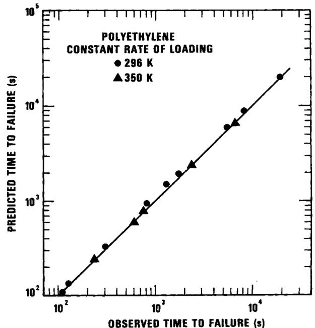
Fig. 4. Prediction of log time to failure at constant rate of loading (based on constant load data) vs log observed time to failure for sample A at two different temperatures. The solid line corresponds to a slope of unity.
