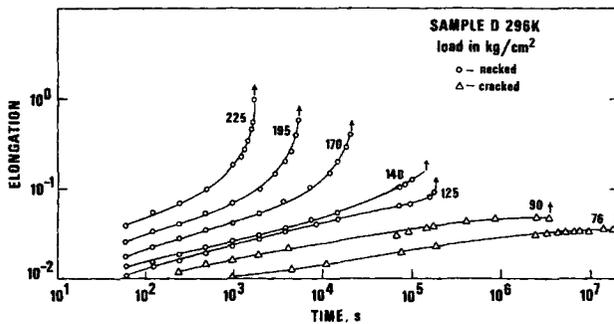
Fig. 6. Log elongation vs log time from creep measurement on sample D. The arrows indicate failure.
