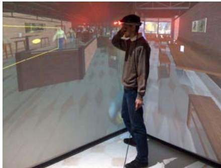
Fig. 3. A user is tracked in a CAVE environment. His position and orientation is used to interact with the characters walking in the virtual environment.
