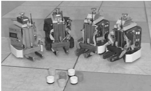
Fig. 1. The R2e robot family: the robots are equipped with a differentially-steerable base, a gripper, piezo-electric bump and gripper sensors used to detect collisions and to grasp pucks, infra-red sensors for collision avoidance, and a radio transmitter for absolute positioning and message passing.
