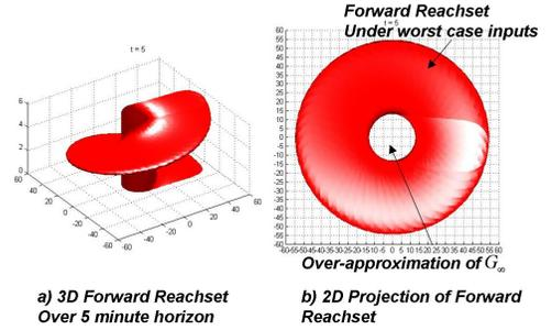
Fig. 3. (a) Forward reachable set computed from unsafe set  $G_\infty$  over time horizon of 5 minutes; (b) projection of forward reachable set onto horizontal plane.
