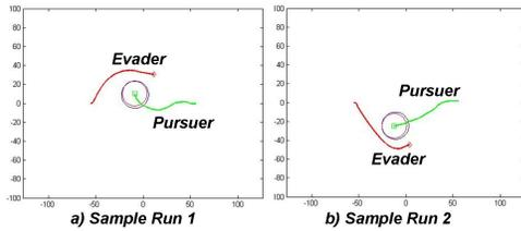
Fig. 6. Trajectory optimization results for random disturbance inputs at nominal path crossing angle  $\phi_0 = \pi$ .
