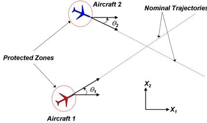
Fig. 1. Two aircraft encounter scenario in horizontal plane.
