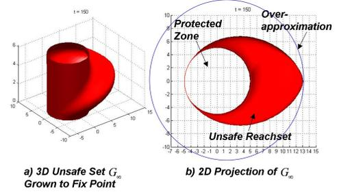
Fig. 2. (a) Backward reachable set for specified input bounds; (b) projection of backward reachable set onto horizontal plane.
