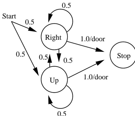
Figure 5.1: A simple Moore machine policy that moves right with probability 0.5, and up with probability 0.5, but stops if the agent has passed through a door. (Arcs are labeled as *probability/variable*, where *variable* can be thought of as a state or observation variable. If there is no variable label for an arc, this matches any variable not already mentioned. In this case, arcs labeled “0.5” match anything other than “door”.)
