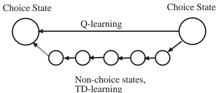
Figure 5.14: Mixed TD and Q-learning. The dashed line indicates that no reinforcement is performed from non-choice states to choice states. Choice state reinforcement is handled by the Q component.
