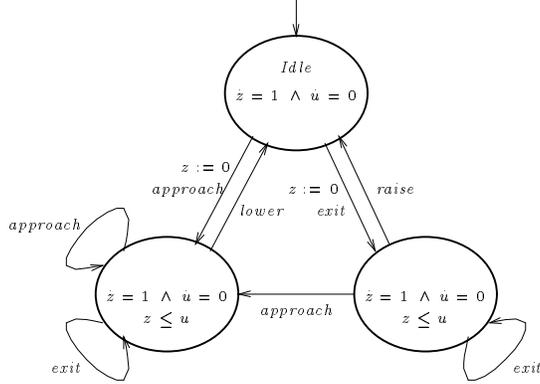
Figure 3: Controller automaton
