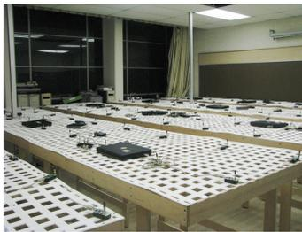
Fig. 10: *NetEye* wireless sensor network testbed
