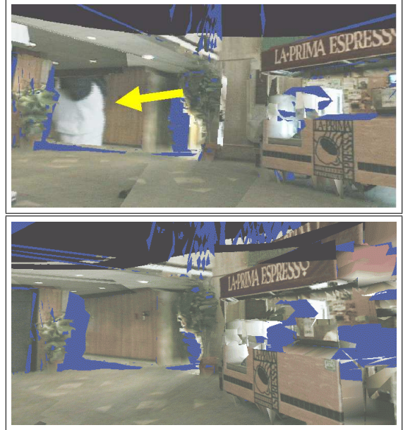
Figure 11: Textured 3d models obtained using Robin. The upper image shows the result without filtering. The lower image shows the resulting model obtained with our algorithm.
