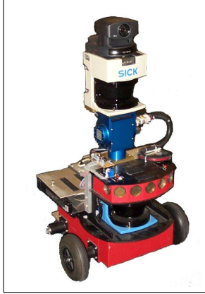
Figure 10: The mobile robot Robin used to generate textured 3d models
