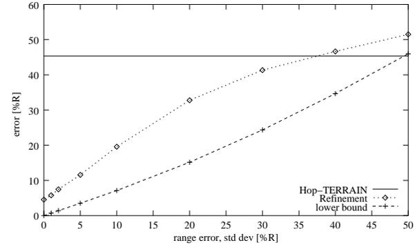
Figure 6: Range error sensitivity (10% anchors, connectivity 12).
