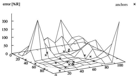
Figure 9: Geographic error distribution (5% anchors, connectivity 12, 5% range errors).
