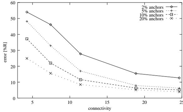
Figure 3: Average position error after Refinement (5% range errors).
