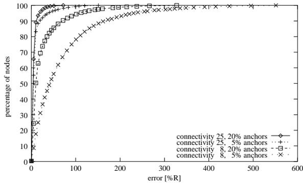
Figure 7: Cumulative error distribution (5% range errors).
