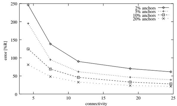
Figure 2: Average position error after Hop-TERRAIN (5% range errors).
