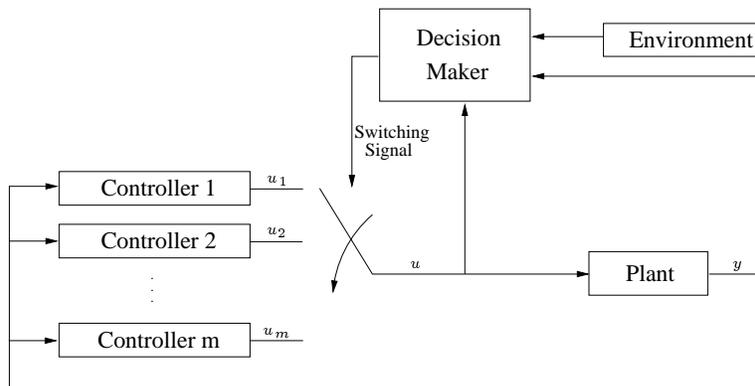
Figure 1: Multi-controller architecture
