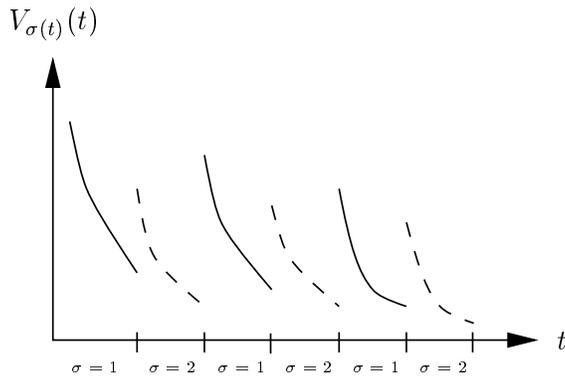
Figure 4: Two Lyapunov functions (solid graphs correspond to  $V_1$ , dashed graphs corresponds to  $V_2$ )
