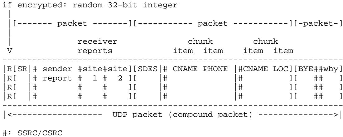
Figure 1: Example of an RTCP compound packet
