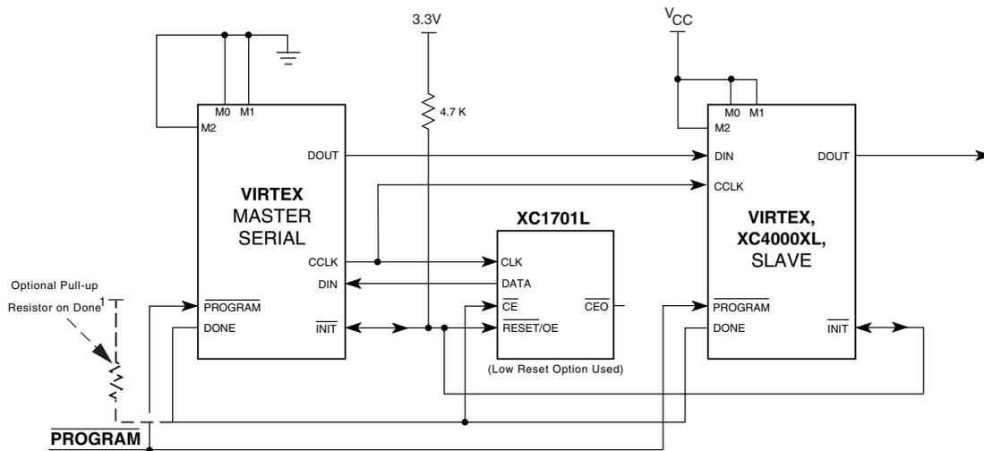
Note 1: If none of the Virtex FPGAs have been selected to drive DONE, an external pull-up resistor of 330 Ω should be added to the common DONE line.
