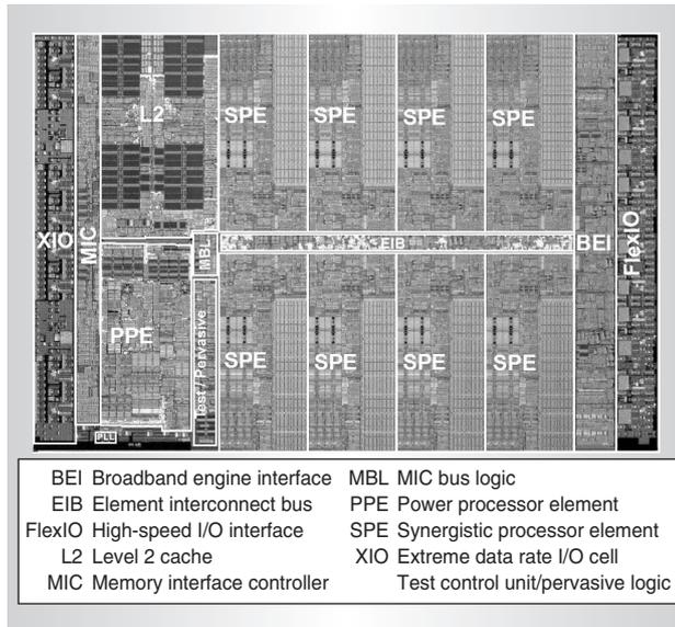
Figure 1. Main functional units of the Cell processor.
