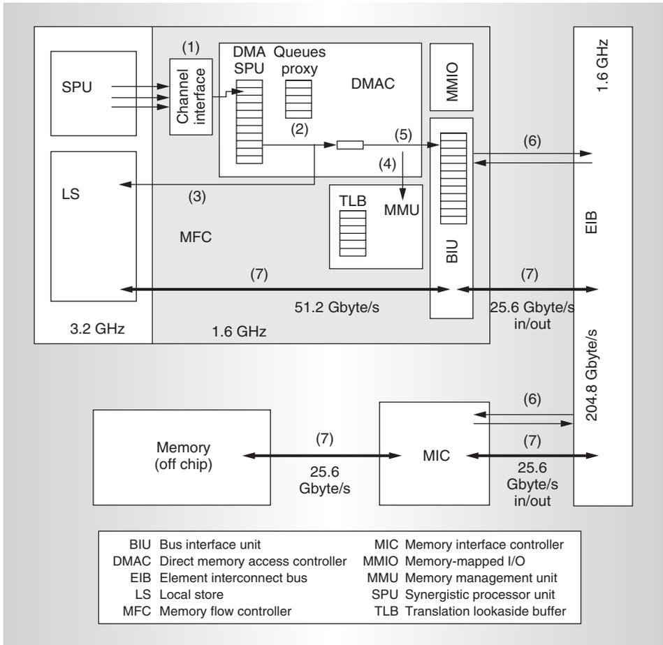
Figure 3. Basic flow of a DMA transfer.
