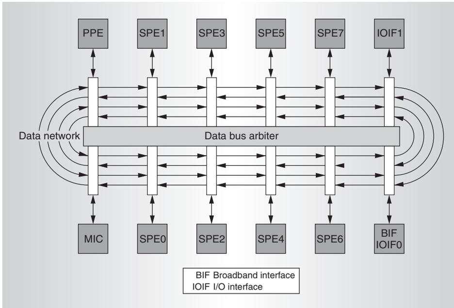
Figure 2. Element interconnect bus (EIB).
