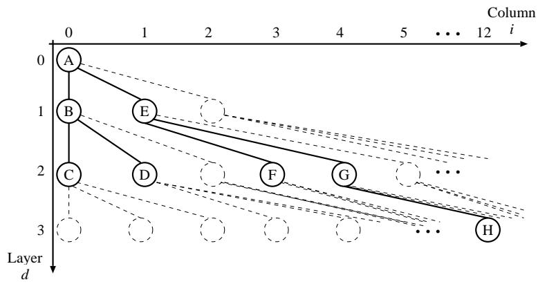
**Fig. 4.** Tree-independent Cartesian node reference system. The syntax tree for the program  $(A (B\ C\ D)\ (E\ F\ (G\ H)))$  is drawn with solid lines. Nodes and links of the maximal tree are drawn with dashed lines.
