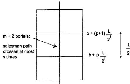
FIG. 3. If a vertical line  $l$  is at level  $i$ , then for  $p = 0, 1, 2, \dots, 2^i - 1$ , the segment of the line between the  $y$ -coordinates  $b + p \cdot (L/2^i) \bmod L$  and  $b + (p + 1) \cdot (L/2^i) \bmod L$  is the edge of a level  $i$  square. It contains a portal at each end and  $m$  other equally spaced portals in between. An  $(m, s)$ -light salesman path must cross this segment at most  $s$  times, and always at one of the portals.
