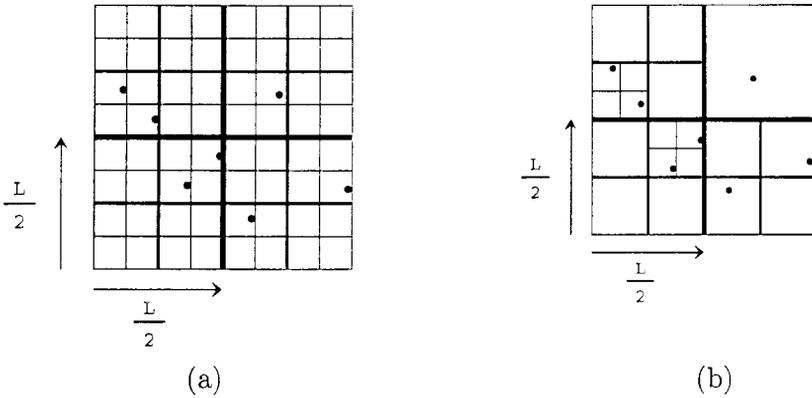
FIG. 1. (a) The dissection. (b) The corresponding quadtree.
