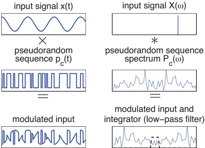
Fig. 2. *Action of the demodulator on a pure tone.* The demodulation process multiplies the continuous-time input signal by a random square wave. The action of the system on a single tone is illustrated in the time domain (left) and the frequency domain (right). The dashed line indicates the frequency response of the lowpass filter. See Figure 3 for an enlargement of the filter’s passband.
