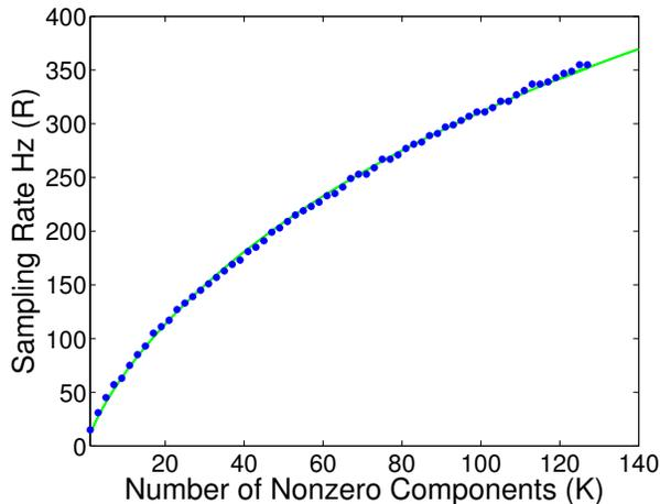
Fig. 5. Sampling rate as a function of sparsity. The bandlimit is fixed at  $W = 512$  Hz. The solid discs mark the lowest sampling rate that achieves successful reconstruction with probability 0.99. The solid line denotes the linear least-squares fit  $R = 1.71K \log(W/K + 1) + 1.00$  for the data.
