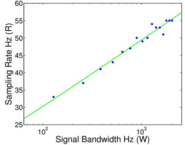
Fig. 4. Sampling rate as a function of signal bandwidth. The sparsity is fixed at  $K = 5$ . The solid discs mark the lowest sampling rate  $R$  that achieves successful reconstruction with probability 0.99. The solid line denotes the linear least-squares fit  $R = 1.69K \log(W/K + 1) + 4.51$  for the data.
