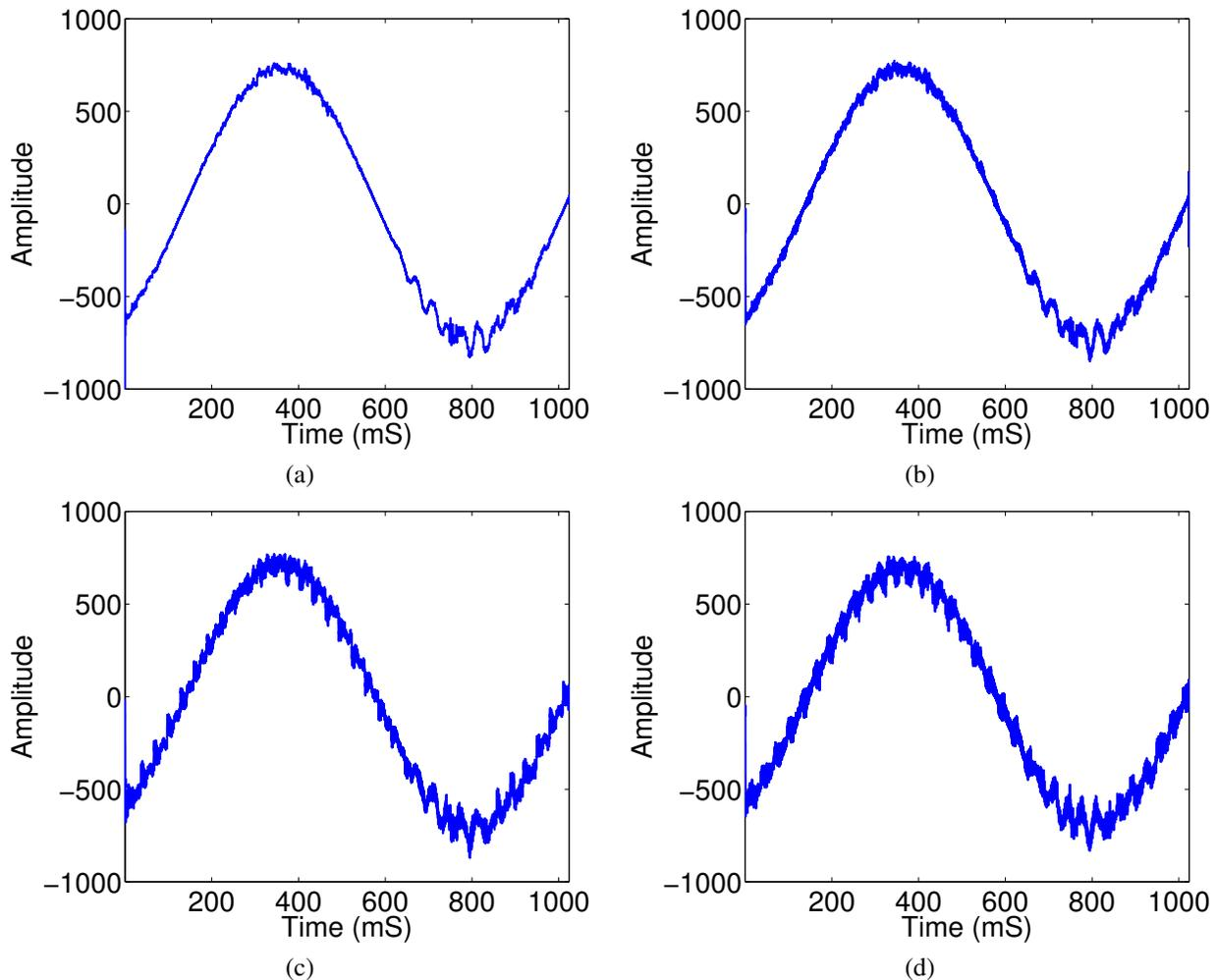
Fig. 7. Simulated acquisition and reconstruction of an AM signal. (a) Message reconstructed from signal sampled at Nyquist rate  $W = 32$  KHz. (b) Message reconstructed from the output of a simulated random demodulator running at sampling rate  $R = 16$  KHz (SNR = 27.8 dB). (c) Reconstruction with  $R = 8$  KHz (SNR = 22.3 dB). (d) Reconstruction with  $R = 3.2$  KHz (SNR = 20.9 dB).
