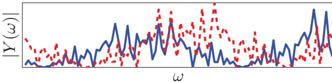
Fig. 3. *Signatures of two different tones.* The random demodulator furnishes each frequency with a unique signature that can be discerned by examining the passband of the antialiasing filter. This image enlarges the pass region of the demodulator’s output for two input tones (solid and dashed). The two signatures are nearly orthogonal when their phases are taken into account.
