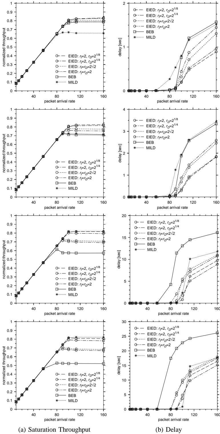
Fig. 3. Simulation results: normalized throughput and delay with respect to packet arrival rate [packets/sec].  $N = 5, 10, 40, 60$ .
