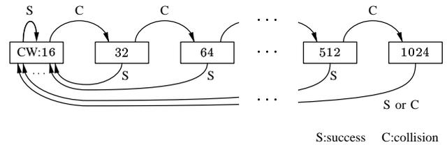
Fig. 1. Backoff mechanism of BEB:  $CW_{\min} = 16$ ,  $CW_{\max} = 1024$ ,  $m = 7$ .
