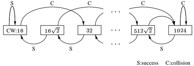
Fig. 2. Backoff mechanism of EIED:  $CW_{\min} = 16$ ,  $CW_{\max} = 1024$ ,  $r_I = 2$ ,  $r_D = \sqrt{2}$ .
