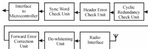
Fig.6 Receiver module flow chart
