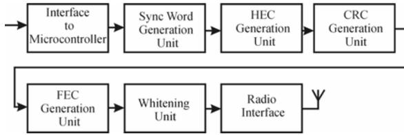
Fig. 5 Transmitter module flow chart
