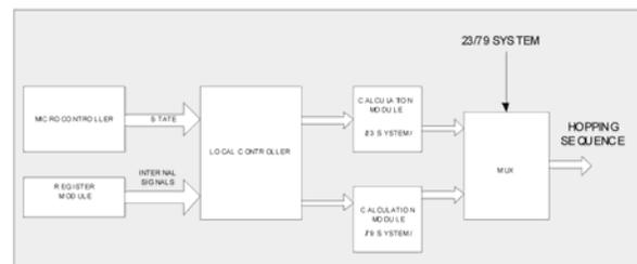
**Fig. 4** Structure of Frequency hopp selection module
