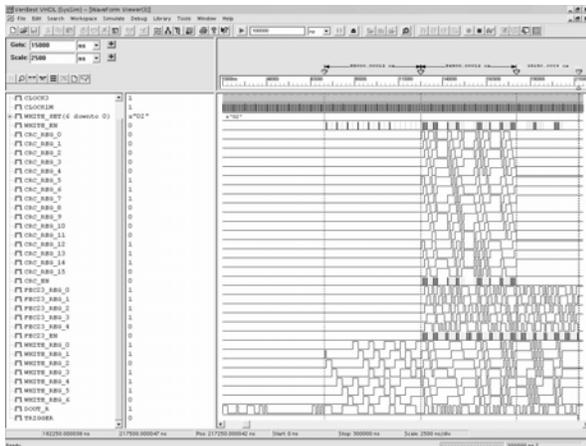
Fig. 15 Post synthesis simulation of transmission of a packet
