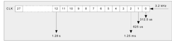
Fig. 7 Structure of Bluetooth clock signal
