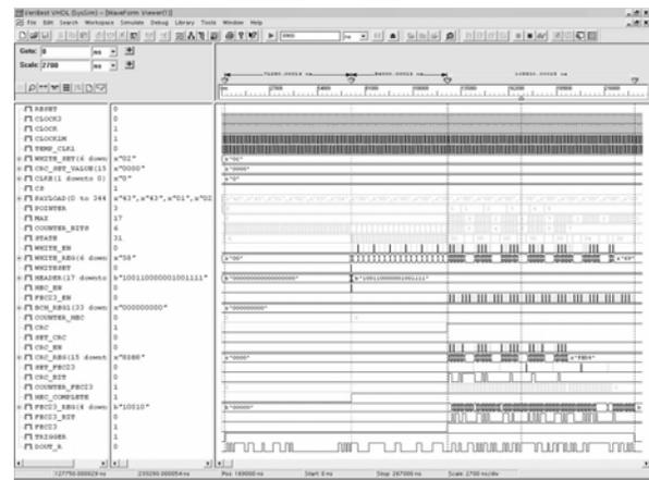
Fig. 14 Post synthesis simulation of transmission module
