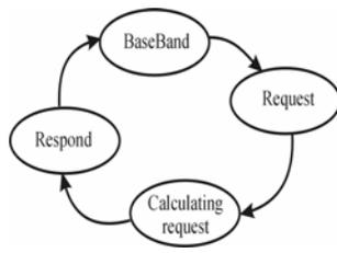
Fig. 9 Structure of LMP layer
