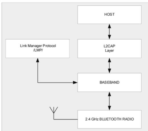
**Fig. 2** Structure of Bluetooth device
