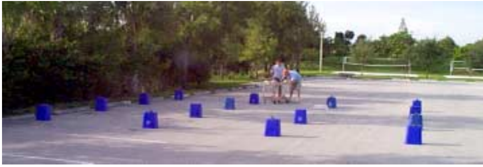
Fig. 8. Parking lot testbed experiment, showing grid of devices, located on top of upside-down recycling bins.
