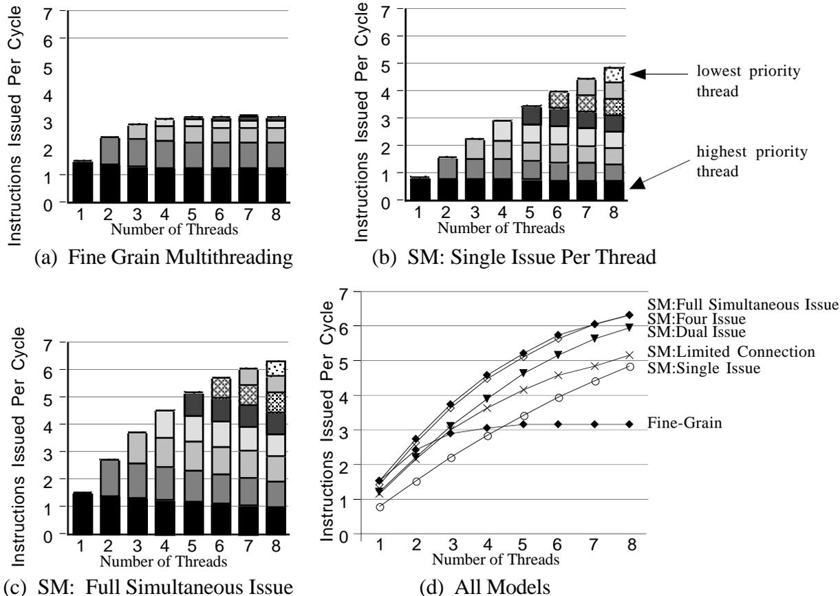
Figure 3: **Instruction throughput as a function of the number of threads.** (a)-(c) show the throughput by thread priority for particular models, and (d) shows the total throughput for all threads for each of the six machine models. The lowest segment of each bar is the contribution of the highest priority thread to the total throughput.
