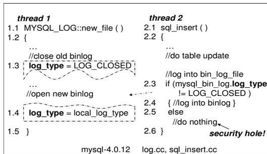
**Figure 5. A real bug from MySQL database server with a case 5 unserializable interleaving: write-write interleaved by a read.** Specifically, the write accesses at lines 1.3, 1.4 are interleaved by line 2.3 read of thread 2. As a result, thread 2 at line 2.3 reads an intermediate value produced by thread 1 and thinks that the log file is already closed. As a result, thread 2’s database action is not recorded in log, which creates a security back door.
