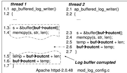
**Figure 4. A real bug from Apache httpd server with case 2 unserializable interleaving: read-read interleaved by a write.** Specifically, the read accesses at lines 1.3, 1.5 are interleaved by line 2.6 write of thread 2.  $buf \rightarrow outcnt$  is read for index update after an append, however its value has already been modified since line 1.3 read. As a result, the server log is corrupted. (there is also a potential case 6 unserializable interleaving between 1.5 and 1.6)
