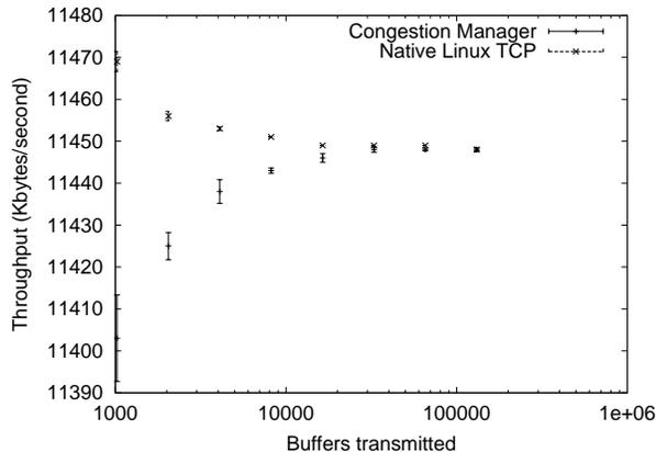
**Figure 4.** 100Mbps TCP throughput comparison. Note that the absolute difference in the worst case between the Congestion Manager and the native TCP is only 0.5% and that the Y axis begins at 11 megabytes per second.
