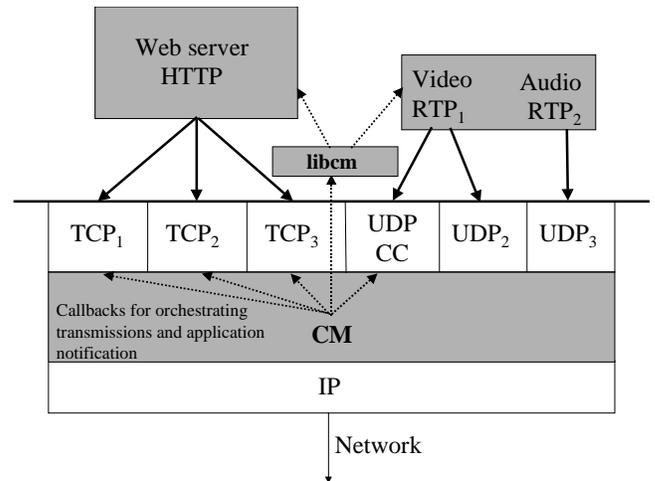
**Figure 1.** Architecture of the congestion manager at the data sender, showing the CM library and the CM. The dotted arrows show callbacks, and solid lines show the datapath. UDP-CC is a congestion-controlled UDP socket implemented using the CM.
