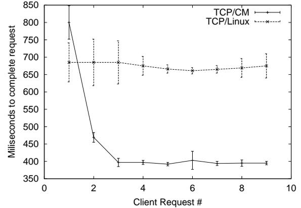
**Figure 7.** Sharing TCP state: The client requests the same file 9 times with a 500ms delay between request initiations. By sharing congestion information and avoiding slow-start, the CM-enabled server is able to provide faster service for subsequent requests, despite a smaller initial congestion window.
