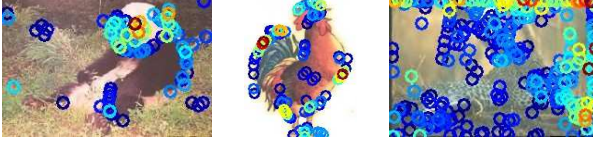
Figure 2. Visualizations of the weights learned by our algorithm for one type of shape feature (geometric blur with 42-pixel radius) for three images from our training set. Each circle is centered at the center point of the feature’s patch and the color of the circle indicates the relative value of the weight. The colors are on Matlab’s jet scale, where dark red is the highest weight (most salient feature) and dark blue is the lowest non-zero weight. Weights that were assigned a zero weight are not shown. Note that the circles are much smaller than the extent of the features and that the colors are scaled separately for each image. For (a), the algorithm learned zero weights for all but 83 of the 400 small geometric blur features computed for the image, and learned that the most important feature is the patch around the eye of the panda. For (b) it learned that the most useful features are on the breast and tail of the rooster, and assigned zero weights to all but 79 of the roughly 400 small geometric blur features. For (c) it learned that the best features aren’t on the leopard at all, but are along the right edge and in the upper-right corner of the image. The Leopards images were drawn from the Corel image set and they have a thin black border around the image that algorithms can exploit, making it a surprisingly easy category.
