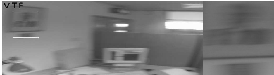
Figure 1: Substantial motion blur due to 2.6 rad/s camera rotation, with 100x100 pixel enlargement
