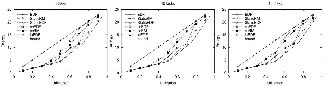
Figure 9: Energy consumption with 5, 10, and 15 tasks
