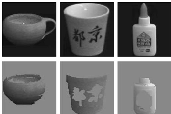
Figure 5. Three images from the COIL database, and the largest non-background component found in each image ( 128 \times 128 color images; algorithm parameters \sigma = 0.8, k = 150 ).
