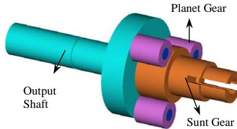
**Figure 11:** Planet Gear Carrier and Sun gear Assembly.
