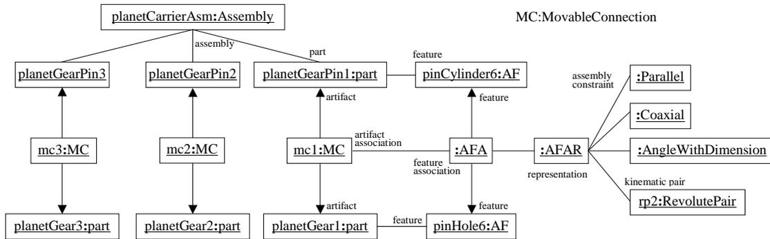
**Figure 10:** Instance Diagram of Planet Gear Carrier Assembly.
