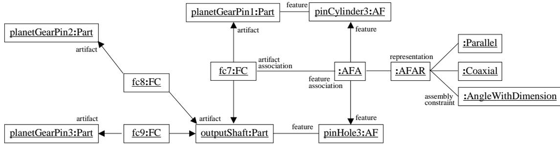
**Figure 8:** Instance Diagram of Planet Carrier Assembly.
