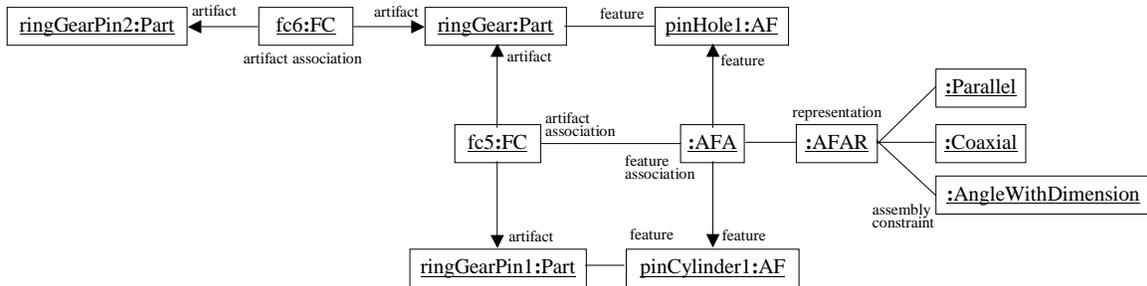
**Figure 6:** Instance Diagram of Ring Gear Assembly.
