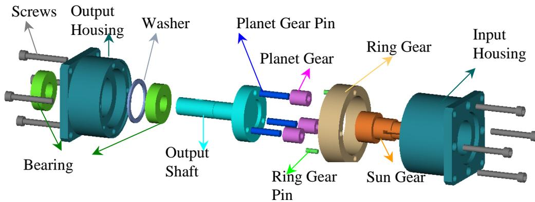
**Figure 3:** Exploded View of the Planetary Gear Model.
