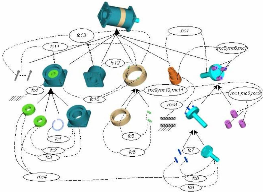
**Figure 4:** Artifact Associations in the Planetary Gear System.
