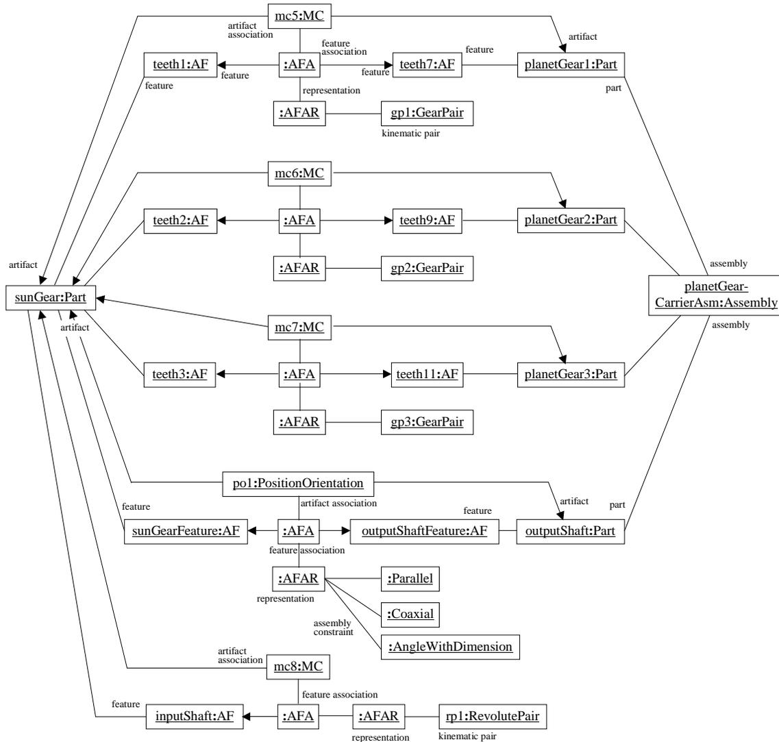
**Figure 12:** Instance Diagram of Planet Gear Carrier and Sun gear Assembly.
