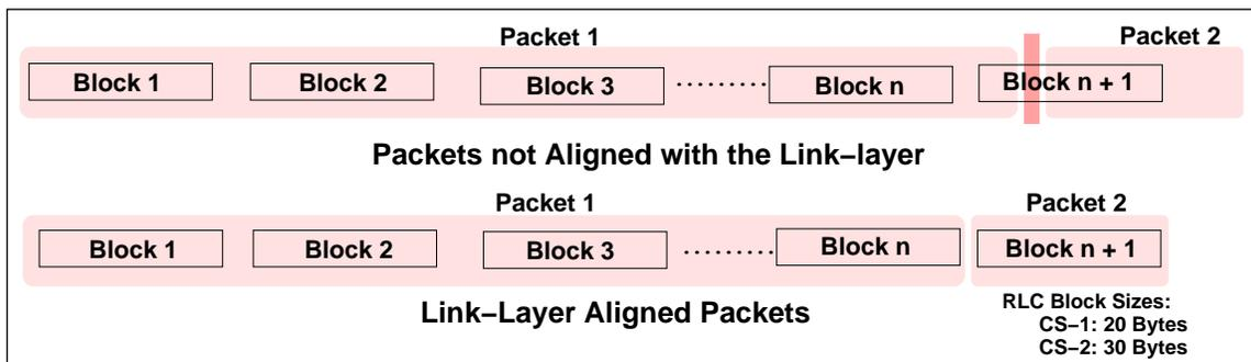
Figure 4. Aligning a packet onto RLC frames.
