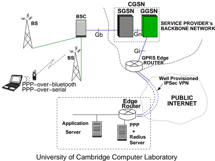
**Figure 1.** The experimental testbed for conducting the GPRS tests. A well provisioned, low latency tunnel transfers all Computer Laboratory GPRS device traffic directly to our PPP server, to which the application server is directly connected via a 100Mbit/s ethernet segment.
