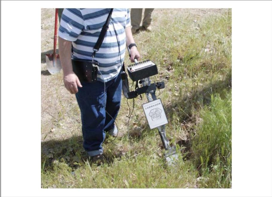
**Figure 2.** The light-weight analyzer for buried remains and decomposition odor recognition (LABRADOR) is an example of a chemical sensing device that was specifically designed for locating chemical scent plumes associated with human decomposition
