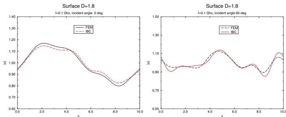
Fig. 19. Modulus of the field,  $\text{rms}h=\lambda/30$
