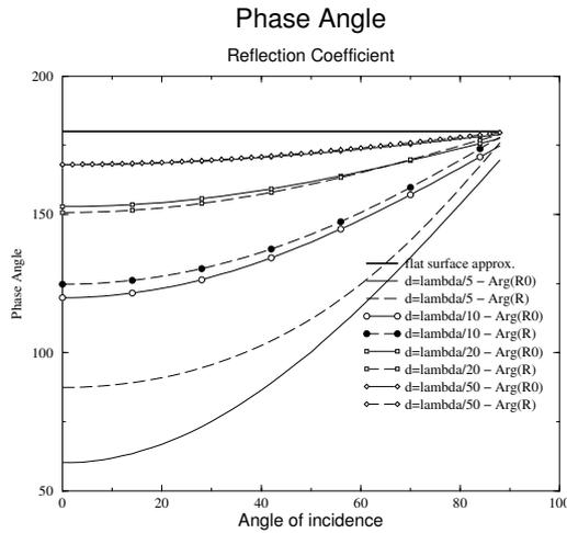
Fig. 5. Phase angle of the reflection coefficient versus the angle of incidence for the sine profile
