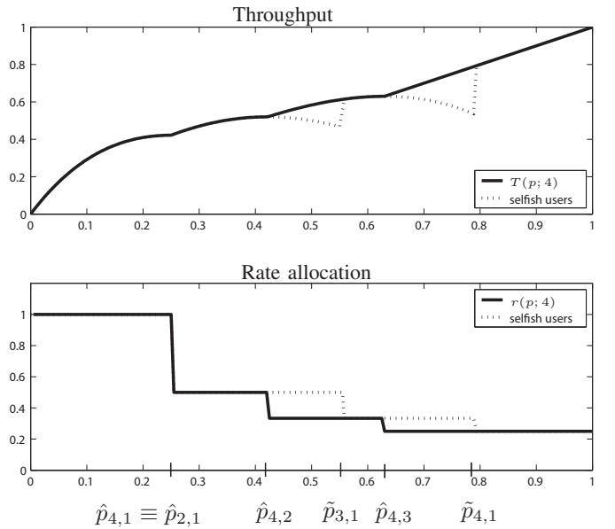
Fig. 3. Comparison between throughput and optimal rate with and without selfish users for a four-user network.
