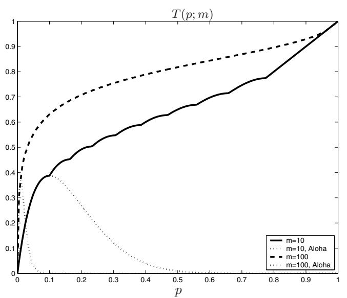
Fig. 2. Comparison between  $T(p; m)$  and the throughput of standard slotted-ALOHA for different values of  $m$ .
