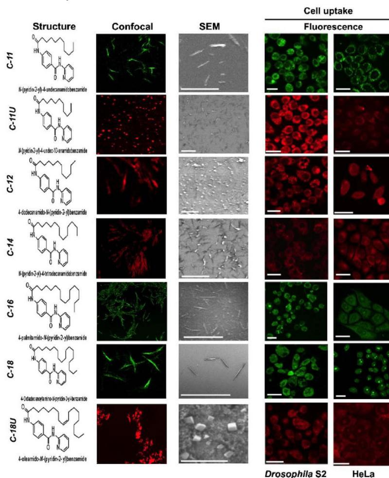
Fig. 2. Physico-chemical properties and microscopic views of 7 PABA nanomaterials. Uptake of several nanomaterials in insect (*Drosophila S2*) and human tumour cells (HeLa) are shown. The differences in chemical structure, shape and surface texture of nanomaterials leads to a variation in cell uptake. Scale- 250 nm (SEM), 50  $\mu$ m (cells) [9].
